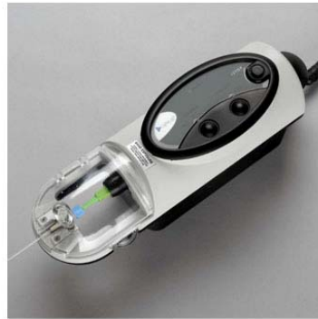
Probe interface unit motor drive unit & motorized pullback unit (1.0mm/sec)
