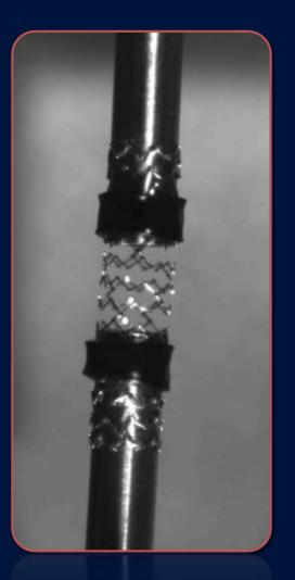
Sequence from high speed video of Fracture Resistance Focal Bend test
