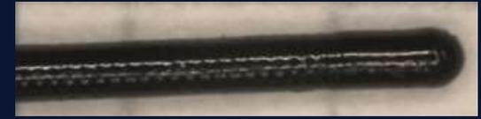
**Polymer jacket wire (polymer coating on spring coil wire)**
