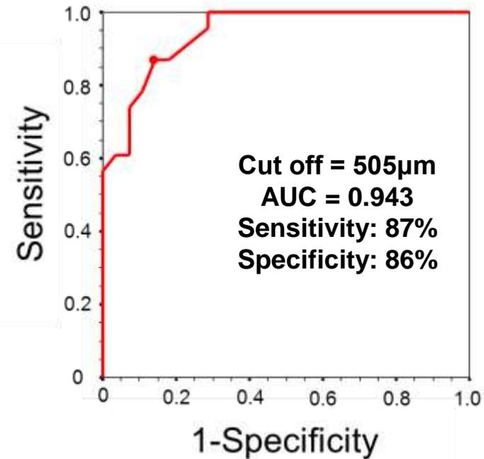
**Conclusion: A calcium plate thickness < 505 μm was the corresponding cut-off value for predicting calcium plate fracture by high pressure ballooning.**
