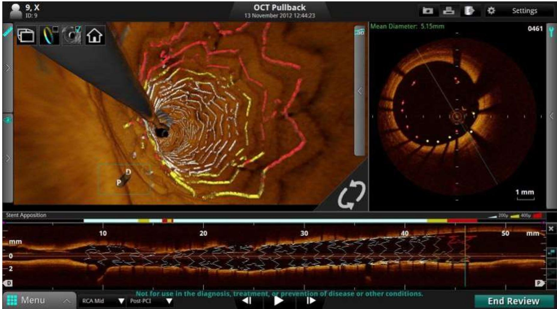
**3-D reconstruction and auto-detection of stent incomplete apposition can be demonstrated as fly through image by new OCT.**
