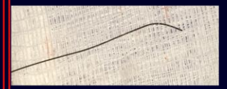
Image 2b: Hi-Torque Command ES wire after attempted reshaping
