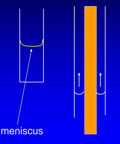
sometimes capillary forces result in misregistration of pressure by the guiding up to 10 mm Hg
