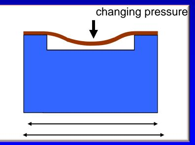
Shrink and expansion of sensor due to changes in temperature and moisture influences pressure on membrane
