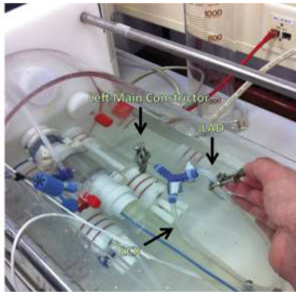
Figure 1. In Vitro Model of the Coronary Circulation
