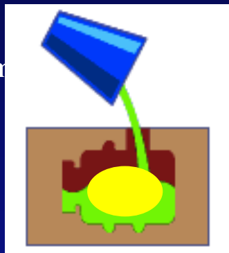
4) Injecting polyurethane material in between the outer and inner molds under the vacuum condition.
