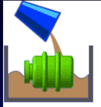
2) Making outer cast with polyurethane.
